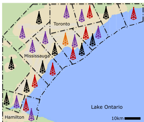
FIGURE 7. A schematic of the Greater Toronto Area and the zones served by the ZSPs deployed by four different IoDSPs each colored differently. Handoff occurs at the boundaries of the zones.
