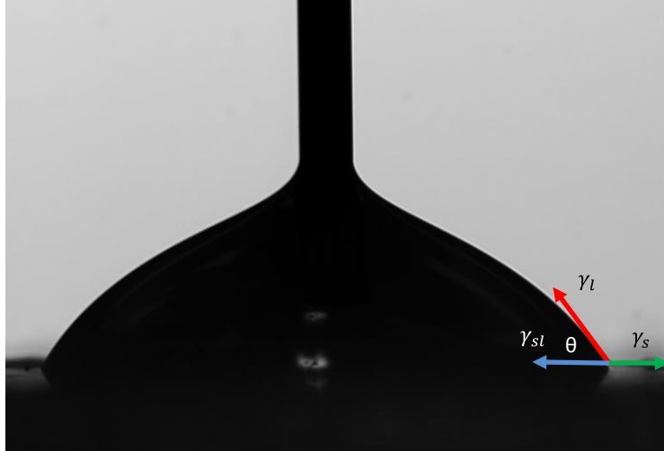
Figure 5-4 Schematic representation of surface/interfacial tensions between a binder drop and polymer-coated glass substrate
