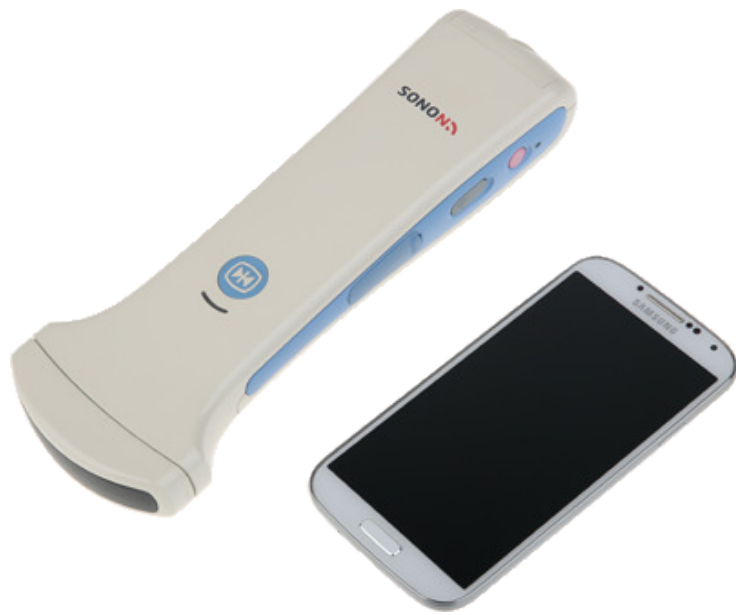
Figure 1.2: A portable ultrasound with mobile phone (Sonon 300C, Healcerion Inc., Korea)
