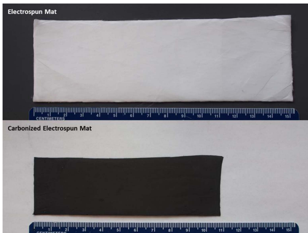
Figure 4. Images of electrospun PAN mat before and after carbonization.
