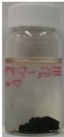
Figure 11. Result of the extraction of oil from oil sands using 60 mg of dodecane instead of toluene. T_{ex} = 50\text{ }^{\circ}\text{C} .
