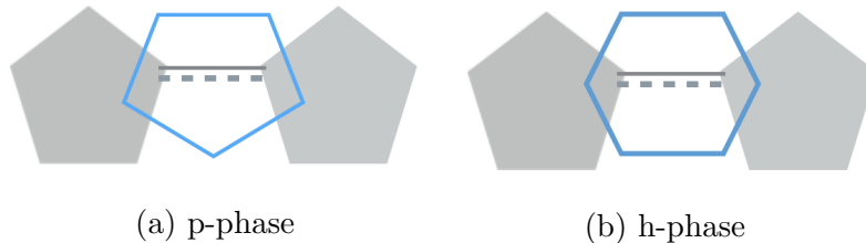
Figure 1.4: A illustration of the p-phase and h-phase relative neighbouring C_{60} molecular orientation: grey part from one cage blue part from its nearest neighbour
