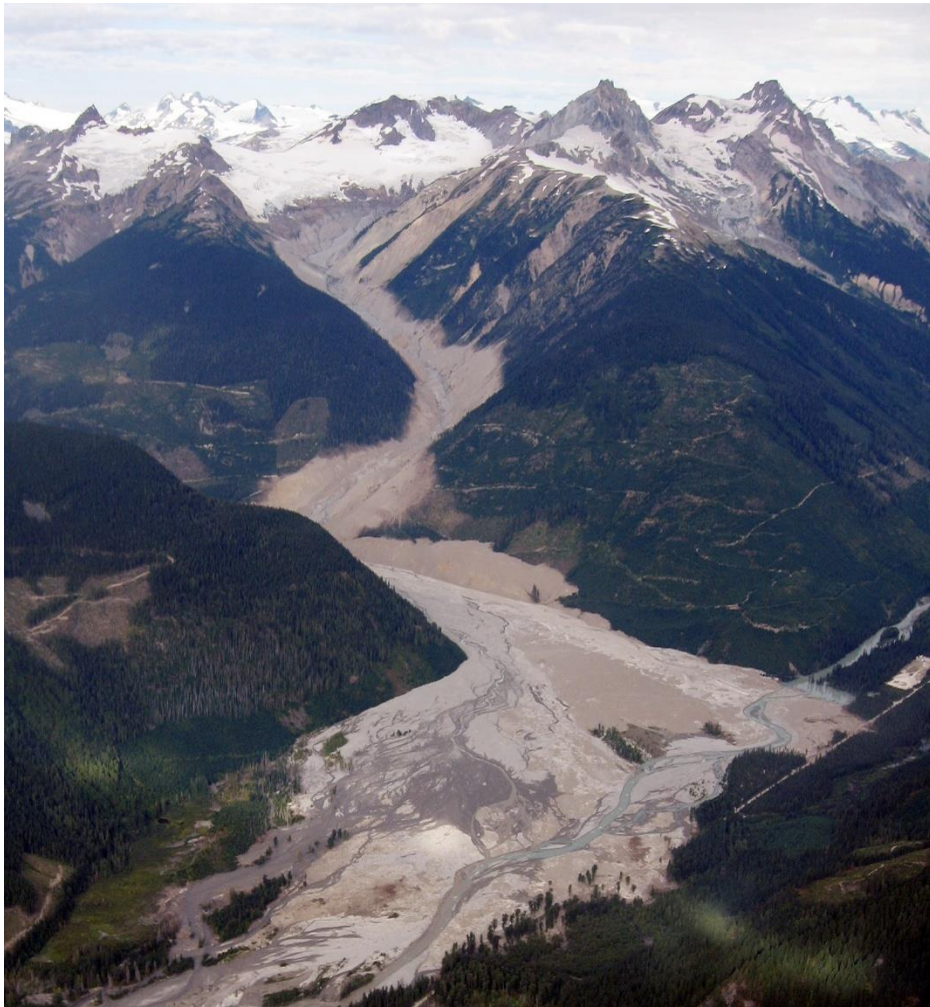
Figure 2.1: Mt. Meager 2010 Landslide (Stephen Evans, Personal Files). This photo illustrates the massive size of the event, with a volume of 48.5 \text{ Mm}^3 , as well as the extensive runout over 12 km long.
