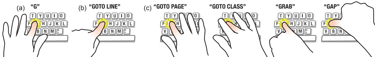
Figure 1.1: Finger-Aware Shortcuts trigger different commands by detecting the finger, hand, and posture used to press the key: (a) for example, pressing G with the left index finger and open hand simply enters the letter “G”; (b) pressing G with the left index and closed hand could trigger a command like “Goto Line”; and (c) pressing G with different right-hand fingers and postures could trigger other commands like “Goto Page”, “Goto Class”, etc.
