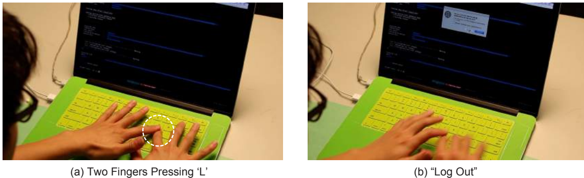
Figure 3.11: Two-Handed Key Press - pressing L with two hands could trigger the uncommon action “Log Out”.
