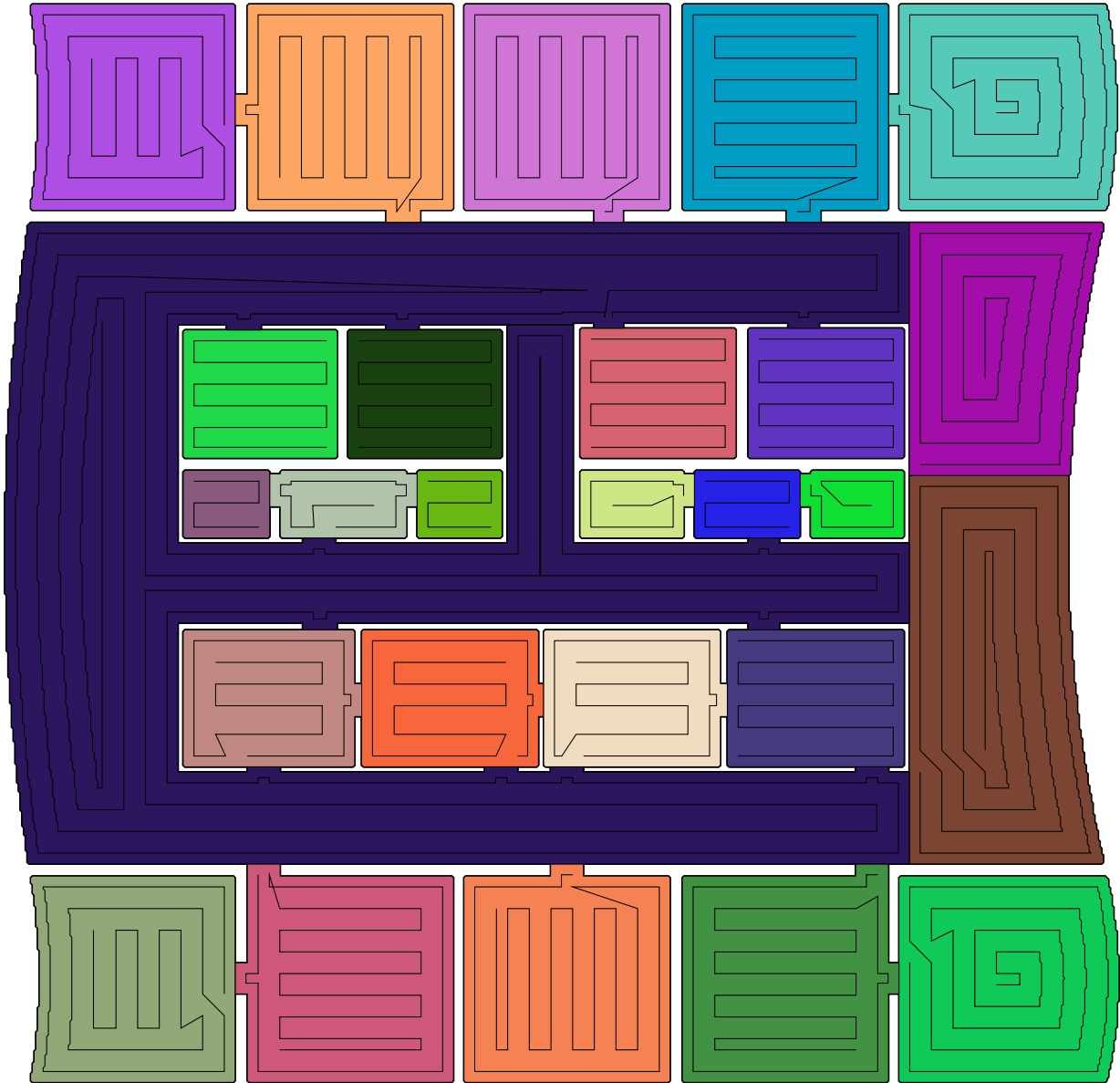
Figure 4.16: CDM Coverage paths generated for Office 2 highlighting coverage in an environment with curved outer boundaries that are approximated as a series of straight line segments.
