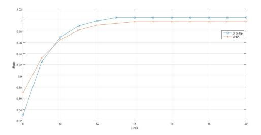
Figure 2.16: Comparing the maximized rates when using superimposed constellation and when control data are placed in the same block as information data
