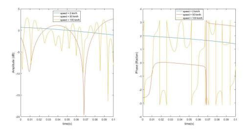
Figure 2.9: Fading channel for three values of mobile velocity
