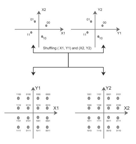
Figure 3.3: Construction of SCMA constellation
