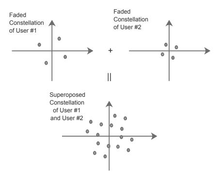
Figure 3.12: Superposition of constellations in multiuser scheme
