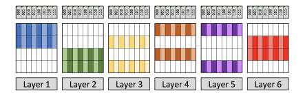
Figure 3.2: SCMA multiuser interference pattern
