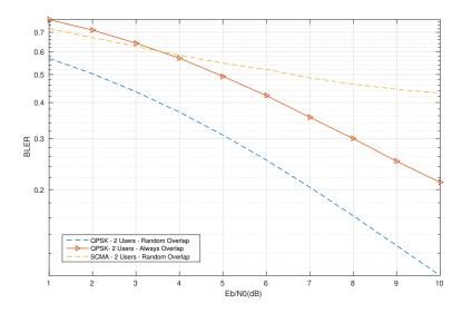
Figure 3.16: Receiver of the multi-user turbo decoder when the users select random tones for transmission (random overlap) and when the users select the same tones (always overlap).
