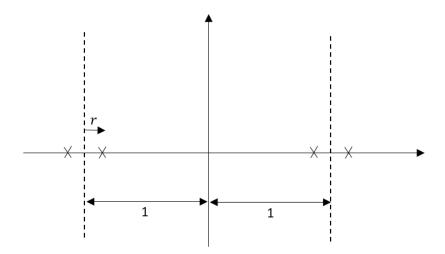
Figure 2.14: Superimposed constellation of control data and information data
