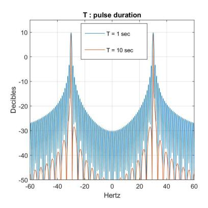
Figure 2.3: FSK signal spectral density
