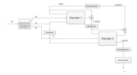
Figure 3.5: Turbo decoder structure
