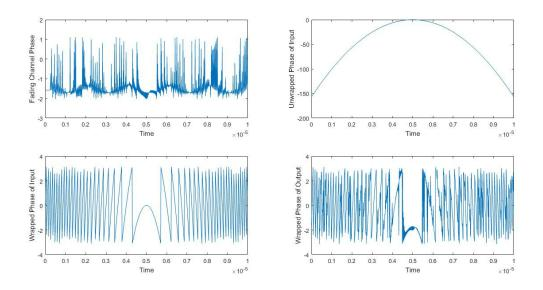
Figure 2.12: Effect of fading channel on 1-bit modulated signal
