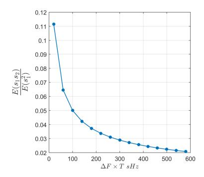
Figure 2.5: Cross-correlation between up-chirp and down-chirp signals as a function of time-bandwidth product
