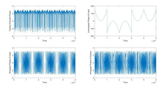
Figure 2.13: Effect of fading channel on 5-bit modulated signal
