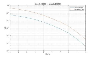
Figure 3.10: uncoded single user SCMA vs. uncoded QPSK
