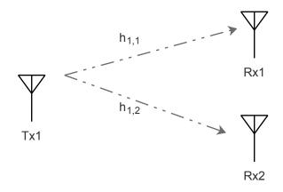
Figure 3.14: Multi Antenna Scheme
