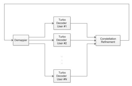
Figure 3.13: Receiver of multiuser turbo decoder
