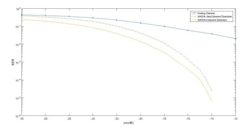
Figure 2.10: Performance of CSS modulation for Fading and AWGN channel
