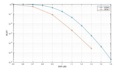
Figure 3.11: BLER of single user scheme in SCMA and QPSK in AWGN chanel
