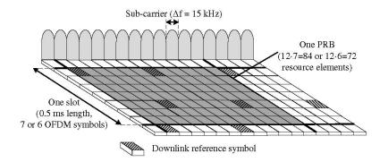
Figure 2.1: LTE physical layer channel resources [2]
