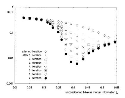
Figure 3.7: Relation between  $I_0$  and BER, illustration from [5]
