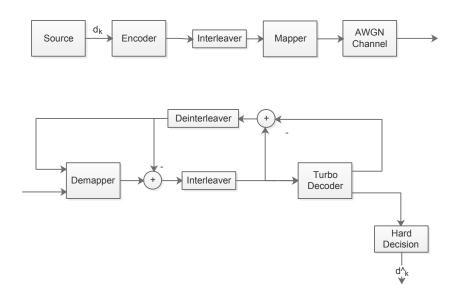
Figure 3.6: Iterative de-mapping system
