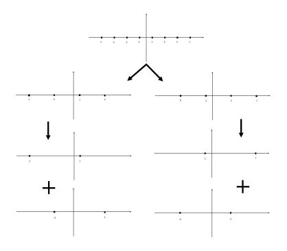
Figure 3.8: Set Partitioning of an 8-point one dimensional constellation
