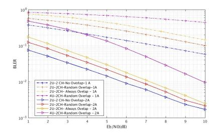
Figure 3.18: Receiver turbo decoder when the users select separate tones, random tones and the same tones for transmission(U, CH, A reperesent user, channel and antennas respectively)
