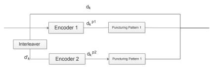
Figure 3.4: Turbo encoder structure
