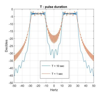
Figure 2.2: Chirp signals spectral density
