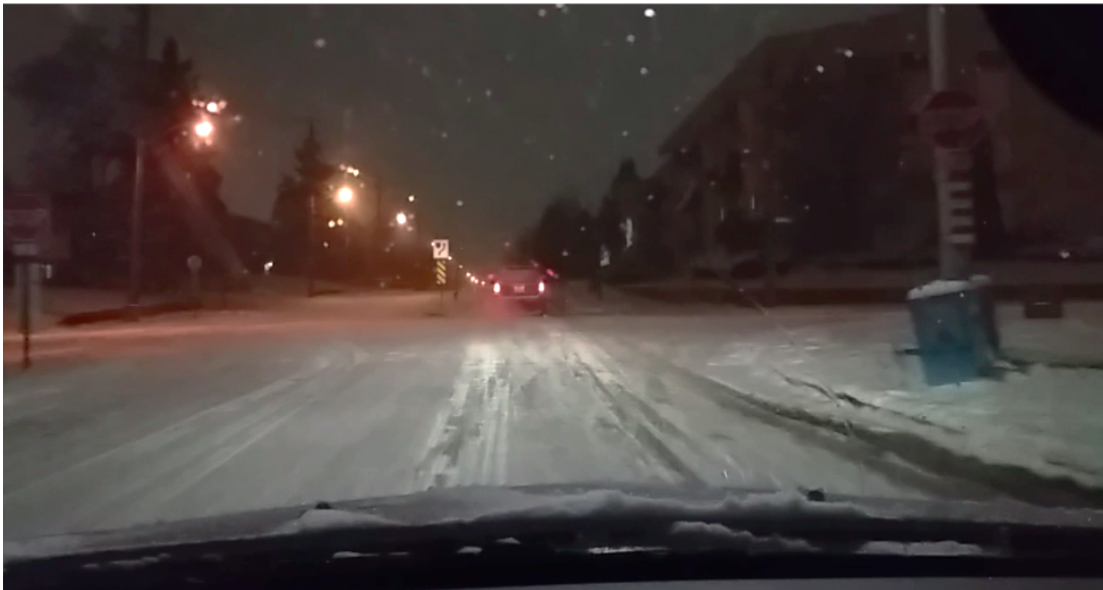
Figure 5.1: Footage captured by pilot project test driver during a slipping event on a snowy road surface, showing elongated tire tracks at the stop sign location
