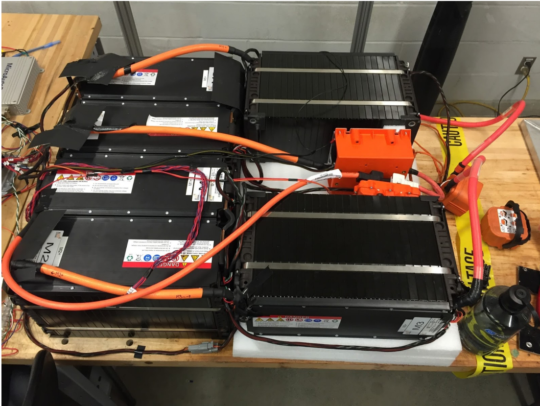
Figure 2.8: 6, LiFePO 4 , A123 battery modules in the configuration used for the UWAFT Camaro test platform
