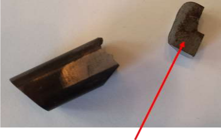
Surface indicating brittle failure
