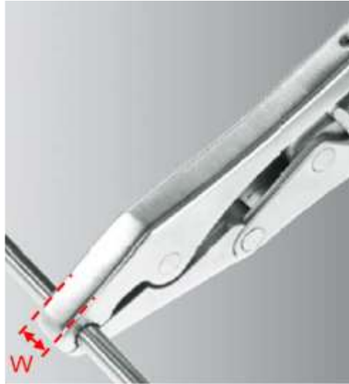
Figure 4.5 Holmed rod clamp ( www.holmed.net ), used to position, rotate and grip onto spinal rods. Gripper contact width W is in the neighborhood of 10 mm. The rod contacting this area should be as straight as possible to ensure adequate grip for adjusting the rod in-situ. This image is used under the fair dealing exception.
