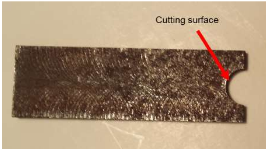
Figure 3.22 Cutting surface of the upper blade of experimental cutter 2
