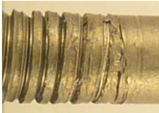
Figure 3.5 Example of cutting disc contact moving along the rod
