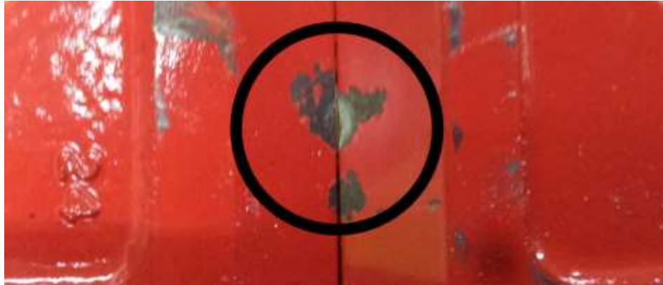
Figure 3.16 Close up view of damage to the cutting blades on the bolt cutters
