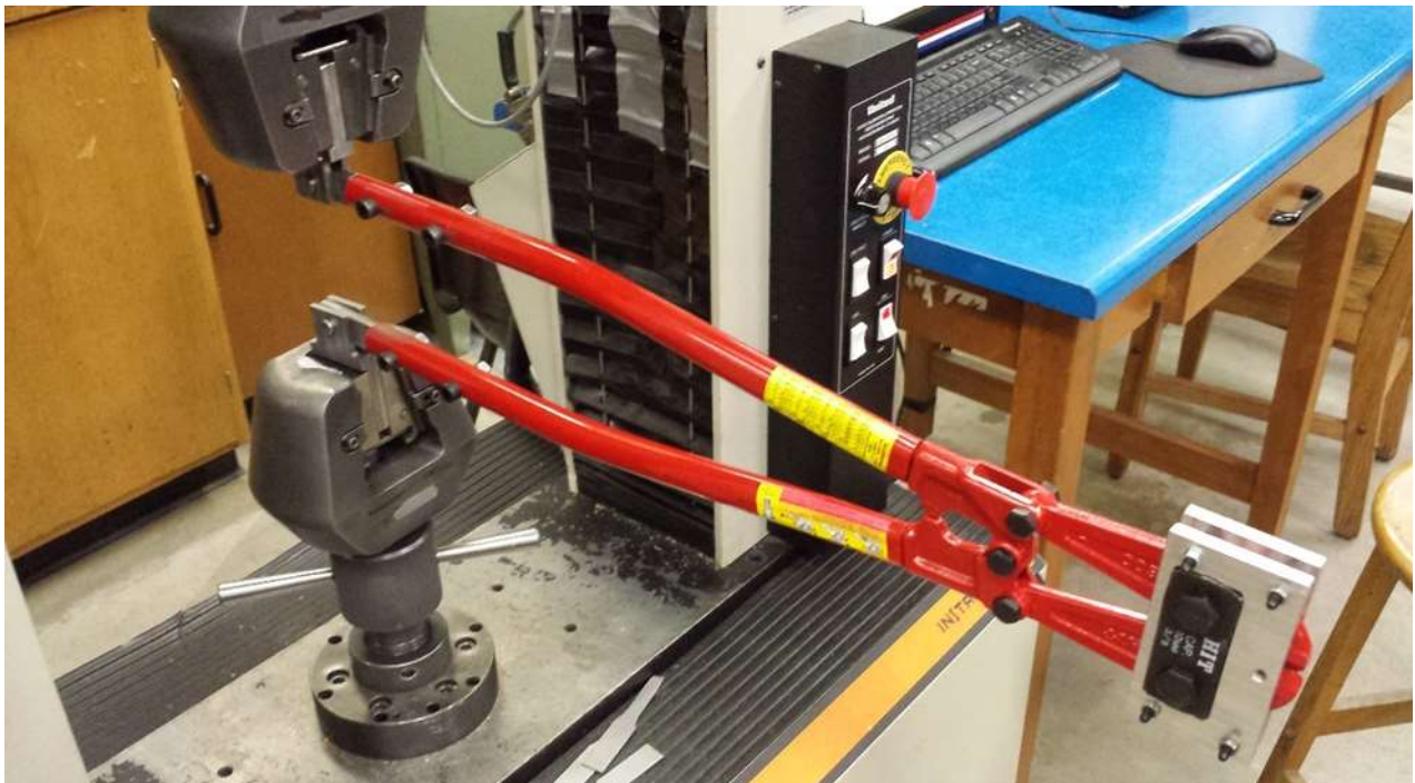
Figure 3.11 Experimental setup for measuring forces required to cut rods using HIT bolt cutter
