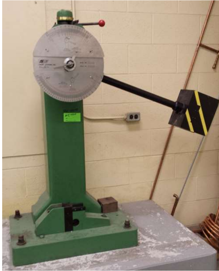
Figure 3.23 Charpy tester, Satec Systems Inc. (Grove City, Pa) Model SI-1K3
