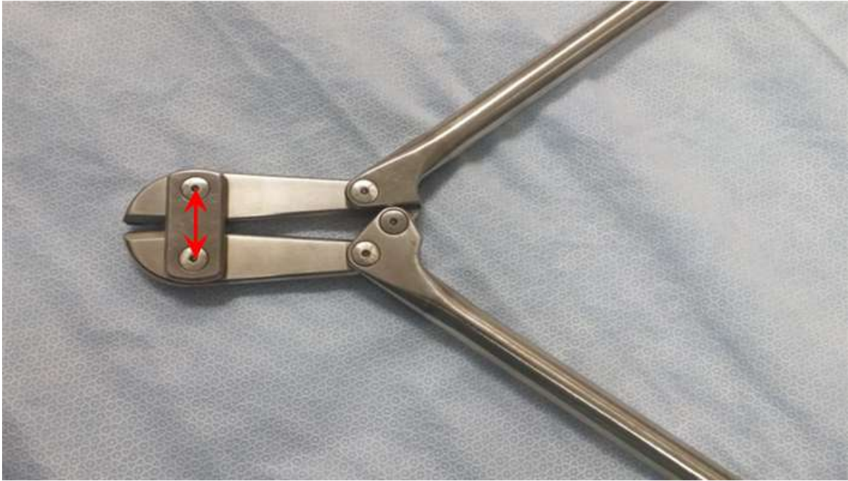
Figure 2.16 Handheld spinal rod cutters for in-situ cutting
