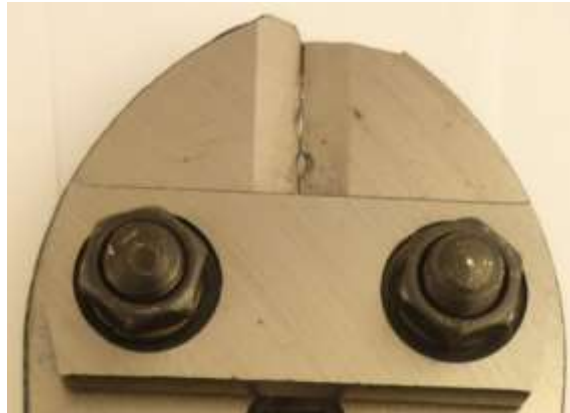
Figure 3.8 Damaged blades of the bolt cutter after cutting the CoCr rod
