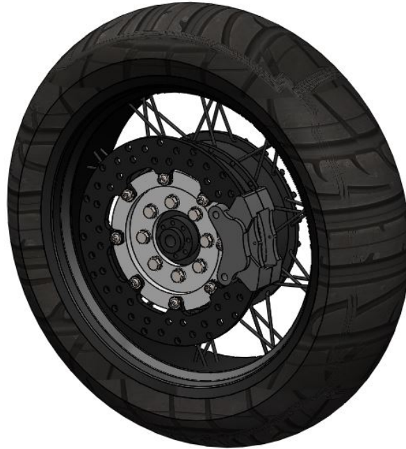
Figure 5.8: Wheel assembly showing the packaging of the selected rotor and caliper. The rotor connects to the wheel via the rotor coupler.
