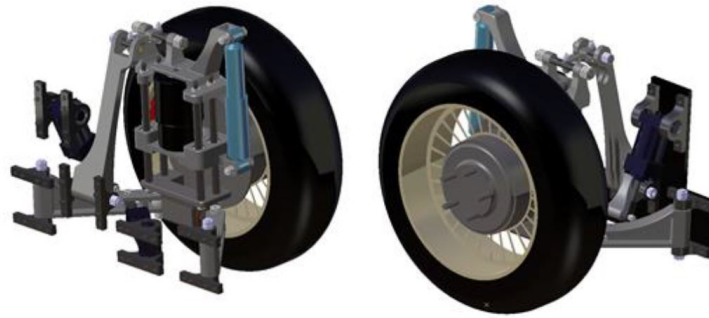
Figure 2.11: The University of Waterloo's corner module developed in the Mechatronic Vehicles Laboratory [30]
