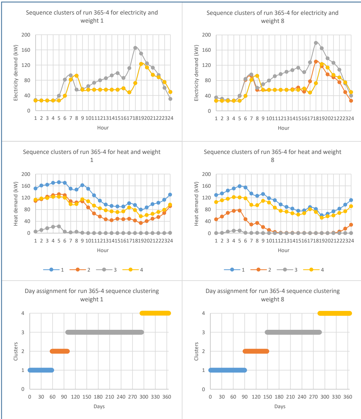
Figure 6-10: Sequence clusters of run 365-4 for heat and electricity with day assignment for weight 1 and 8
