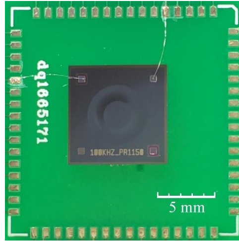
Figure. 5.3.1 A photograph of the fabricated annular-cell CMUT on a PCB carrier.
