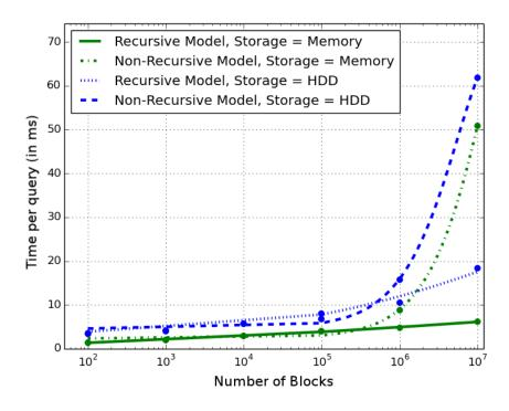
Figure 5.1: Representative result. Shows the number of data blocks vs. time per request, with data blocks of size 1 KB. We use ZeroTrace with a PathORAM schema and the storage is HDD. We use a tree top caching mechanism which caches all the recursion and integrity trees and all but the last level of the data tree.
