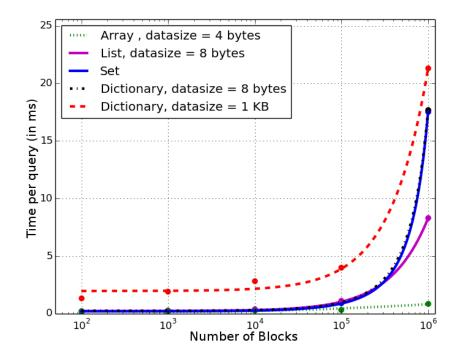
Figure 5.7: Evaluation of our oblivious memory controller library for Set/Dictionary/List/Array. Array is a direct call to our core memory controller, which uses ORAM recursion to be asymptotically efficient.
