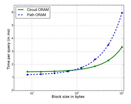
Figure 5.6: Evaluation of ZeroTrace comparing PathORAM and CircuitORAM as the underlying ORAM schema for varying data block sizes with  $N = 10^7$
