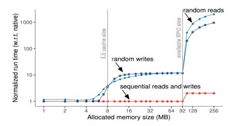
Figure 3.1: Normalized overhead of memory accesses with SGX enclaves. (Figure 3 from Scone by Arnautov et al.[3].)
