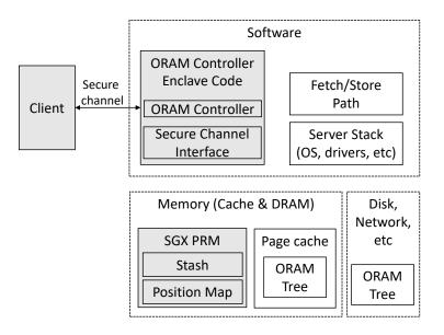
Figure 4.1: System components on the server. Trusted components (software and regions of memory) are shaded. Depending on the setting, the client may be connecting from a remote device (not on the server) or from another enclave on the same machine.
