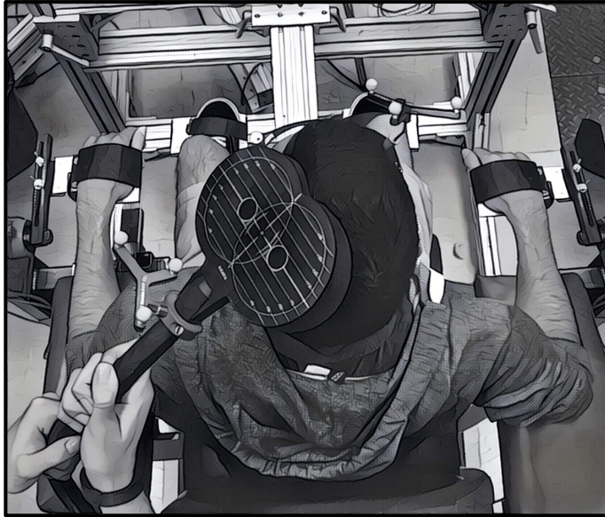
Figure 4.1. Experimental set-up for Experiment 1 and 2. Overhead view of the experimental set-up where subjects were instructed to perform isometric contractions [both ipsilateral (left upper and lower limb) and contralateral (right upper and lower limb) to stimulation] while they were secured in manipulandums. The right ECR (muscle of interest) was at rest in all experimental conditions. Please note: during Experiment 1 more custom build manipulandums were required to secure the various upper and lower extremity muscles that were tested.
