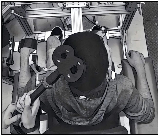
Figure 5.1. Experimental Setup. Overhead view of the experimental set-up where subjects were instructed to perform isometric contractions of their left wrist extensors and/or right dorsiflexors while they were secured in manipulandums. The right ECR (muscle of interest) was at rest in all experimental conditions.
