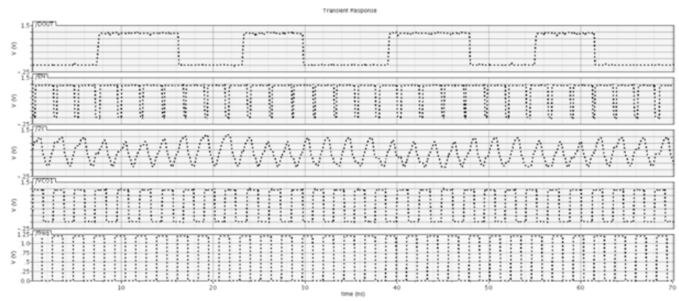
Figure 5.21: Cadence timing waveform simulation showing digital output of 2nd order Sigma Delta TDC with a sampling frequency of 450 MHz
