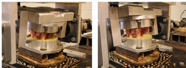
Figure 2. Images of a specimen in the material testing system: specimen in flexion (left) and extension (right). The moment angle data were sampled from an independent servomotor connected in series with a torque cell.
