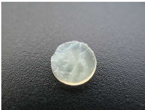
Figure 3. Ciprofloxacin precipitate on the surfaces of DMAA TRIS + HA 35 kDa disc.
