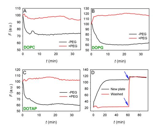
**Figure 5**. (A) Fluorescence signal of Rh-labeled DOPC (A), DOPG (B) and DOTAP (C) liposomes with and without 0.01% PEG 20k. (D) Fluorescence signal of calcein encapsulated DOPC liposomes in a new surfactant coated plate (black trace) and after washing with ethanol and PEG (red trace). The arrow heads indicate the time when Triton X-100 was added.
