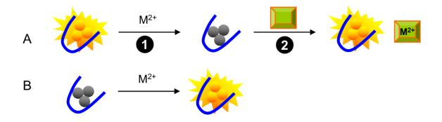
**Figure 6**. (A) Detection of heavy metal ions that can quench the fluorescence of DNA-templated AgNCs (step 1). If this reaction is reversible, addition of a metal chelator might recover the quenched fluorescence (step 2), allowing the detection of the chelator. (B) In some cases, non-fluorescent NCs show fluorescence enhancement upon addition of heavy metal ions.
