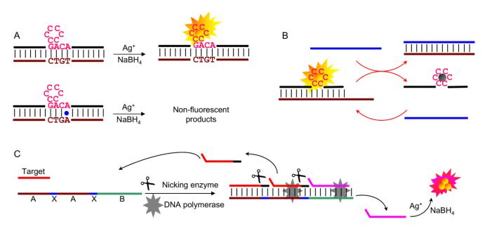
**Figure 4**. (A) A duplex DNA containing a C<sub>6</sub> bulge can template fluorescent AgNCs, while the synthesis is hindered by the presence of a single base mismatch. (B) The fluorescence of AgNC in the bulge can be modulated by hybridization and removal of the cDNA. (C) A DNA machine method to generate a DNA template for making AgNCs.
