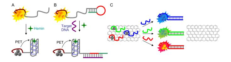
**Figure 3**. Molecular beacon type of signaling method involving an external quencher. (A) Hemin/DNA complex can quench AgNCs. (B) DNA detection using hemin as a quencher. (C) Multiplexed detection of DNA using AgNC probes on GO. For clarity of the figure, the oxygenated species on GO is not drawn.
