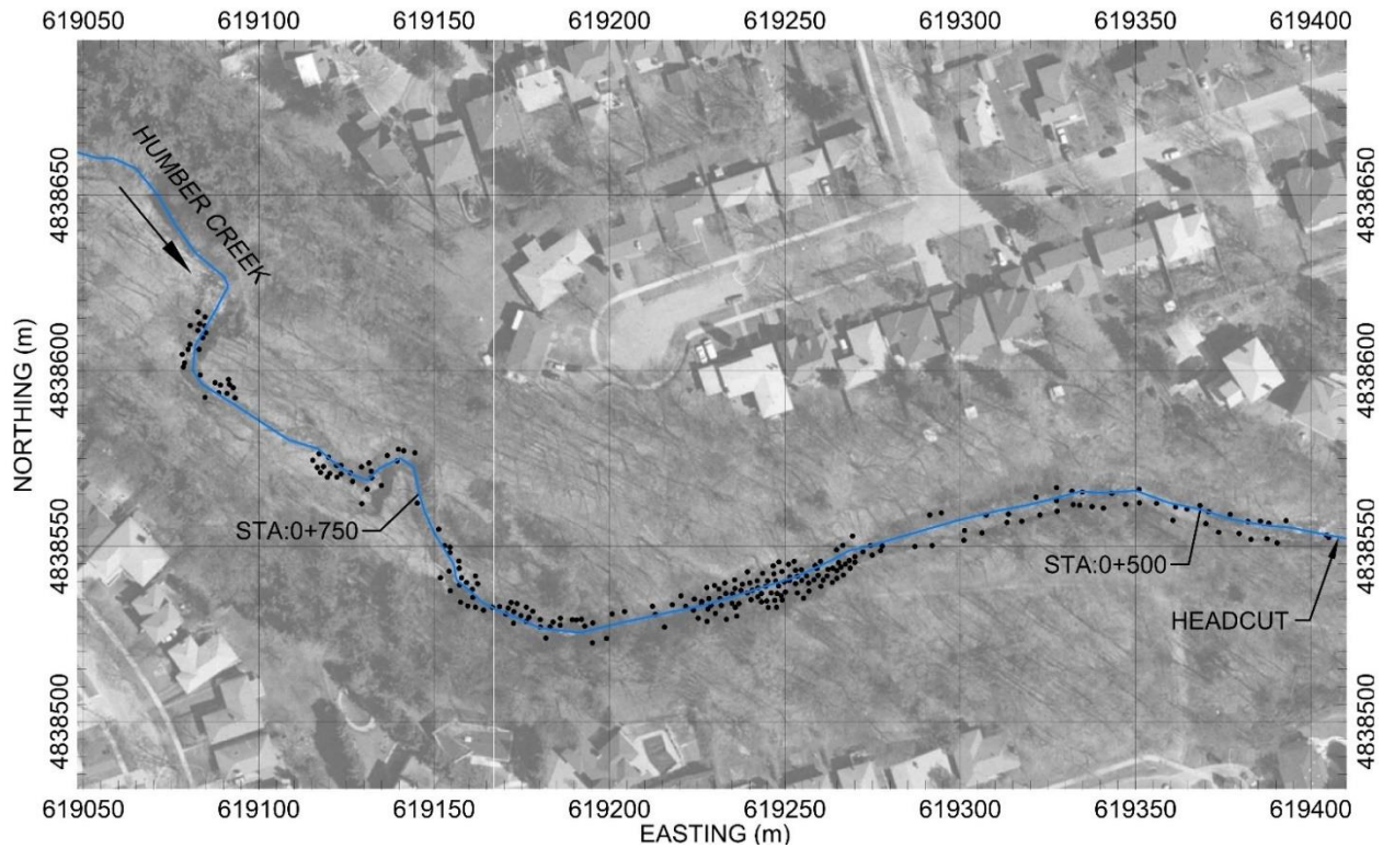
Figure 4 - Spatial distribution of particles seeded with PIT tags (black dots) in Humber Creek. 50 m grid lines shown.
