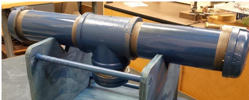
Figure 26: Custom absorption cell fabricated from steel piping components with 1.5" sapphire windows and three ports to be used as inlets or outlets to the cell.
