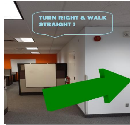
Figure 2. Screenshot of the indoor augmented reality navigation aid application while being assessed at the test location. The augmented arrow and text are visual instructions displayed on the screen of the devices. The application also provides voice instructions that tell the user the same instructions as visible on the screen. The same interface was deployed on both digital devices used in the experiment.
