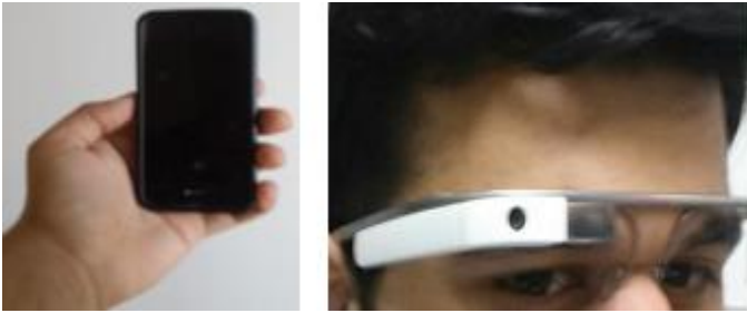
Figure 1. The figure describes how the two navigational devices would be physically operated for indoor navigation. The wearable device on the right (i.e. Google Glass) works as a head mounted display where the information is received on the augmented reality screen focused on the pupil of the right eye. The smartphone on the left needs to be positioned in an upright position for appropriate orientation.
