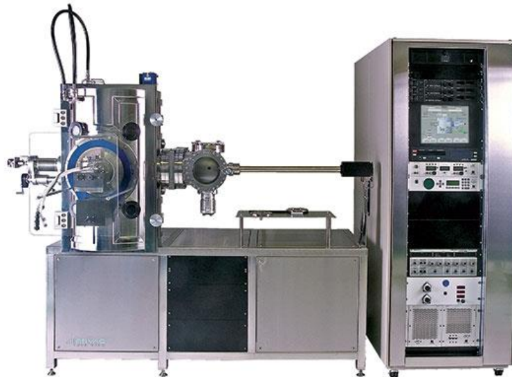
Figure 2.1 The picture of a modern evaporator for R&D purpose. (Picture courtesy to the Intlvac Thin Film Corporation) 2
