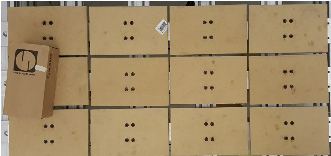
Figure 4.3: Package is pulled with a string along the weighing grid.
