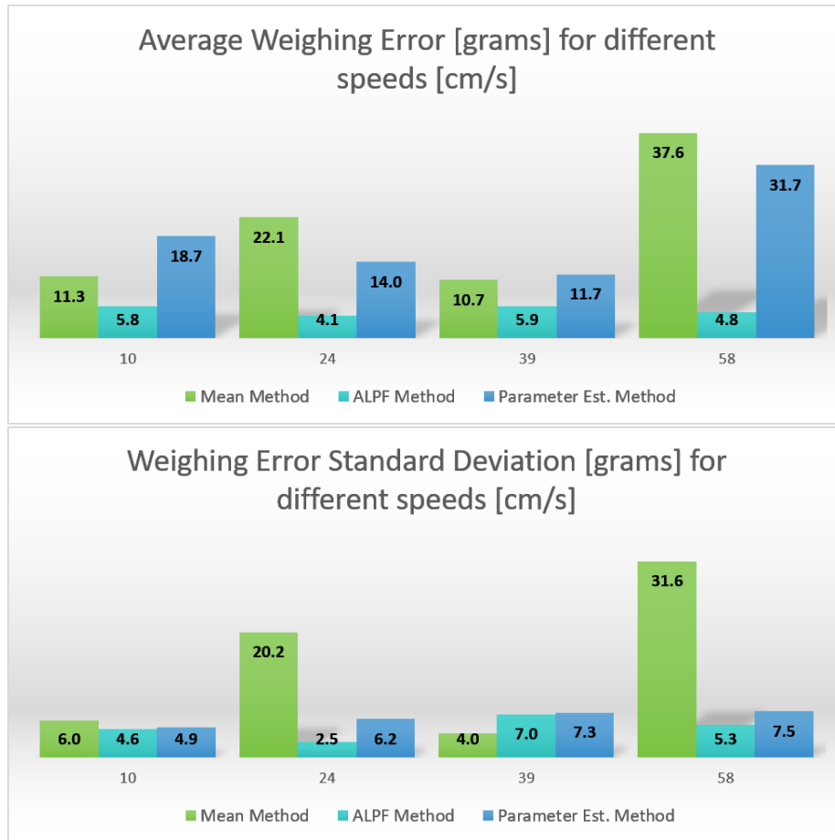
Figure 4.7: Experiment 1: weighing error for the three filtering methods at different speeds.
