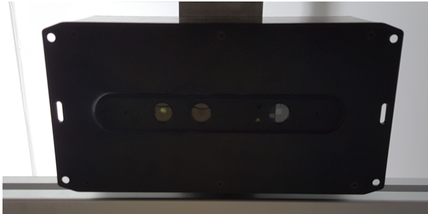
Figure 2.32: Object detecting and dimensioning vision system.
