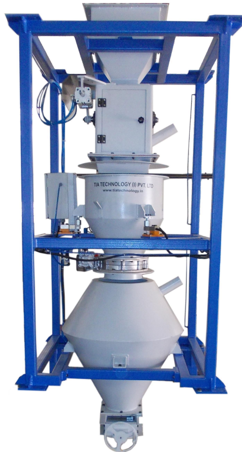
Figure 1.7: Material Totalizing Batch Weigher [12]. © 2014 TIA Technology Pvt. Ltd.
