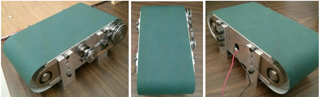
Figure 2.26: Prototype for the first iteration of conveyor belt design.
