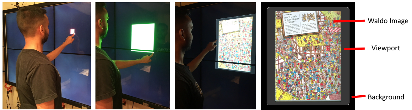
Figure 1. A participant in front of the 4 \times 1.2\text{m} display. Viewports were initially created by drawing their diagonal with a single touch point. Viewports smaller than 400 \times 400 px were not allowed, indicated by a red viewport on the display (Panel 1). Once the viewport exceeded this size it was displayed as green (Panel 2), at which point participants could release their touch to create an initial viewport (Panel 3). The contained Where’s Waldo image was sized to maximize its area within the surrounding viewport (Panel 4).
