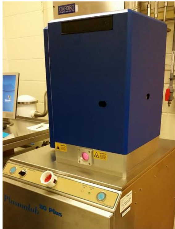
Fig. 5.3: Plasmalab Oxford PECVD in our lab used for SiN deposition.
