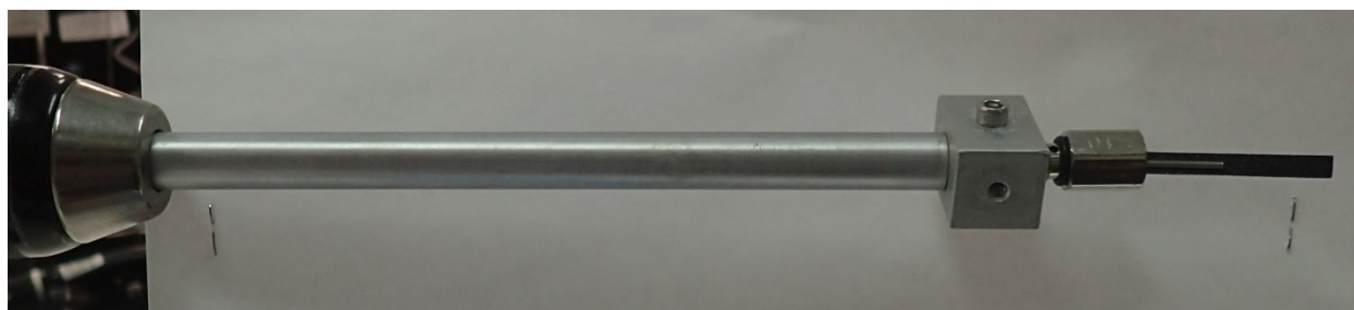
Figure 1. Modified power drill set-up holding a 4 cm x 5 mm DVB/PDMS/Carbon mesh TFME membrane
