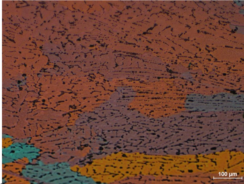
Figure 68: PSC sample grain structure for a PGN sample deformed at 300 °C and strain rate of 10 up to a strain of 0.5, heat treated with schedule H3 and annealed at 500 °C for 12 hours.
