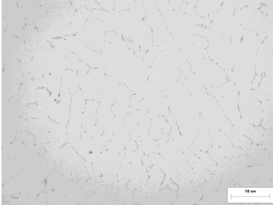
Figure 30: As-polished PGN sample after homogenization schedule H3
