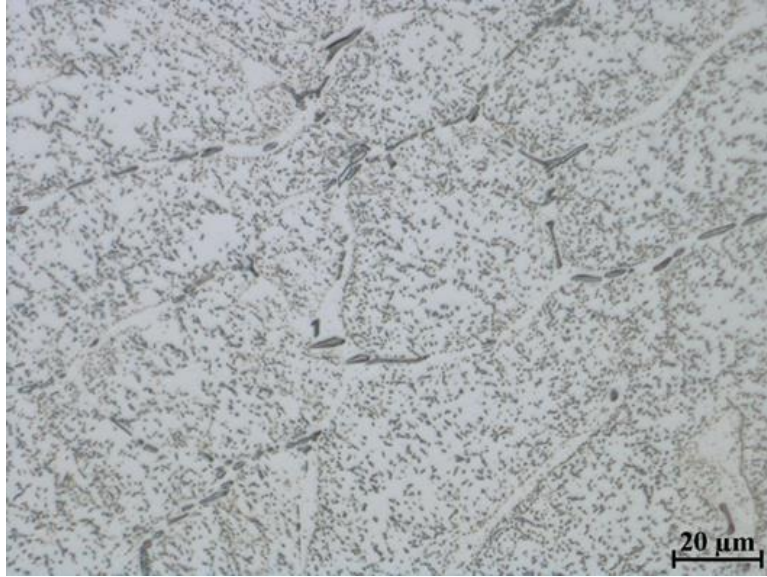
Figure 49: Optical micrograph of PGN alloy after homogenization of H1
