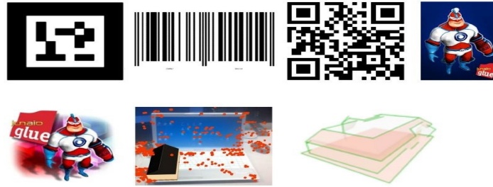
Figure 1.1.: This figure represents the different trackables that can be utilized to overlay virtual imagery. The trackable include fiducial ID markers, barcodes, QR codes, image based markers, borderless marker, 3D point map, and CAD edge model (Koch, Neges, König, & Abramovici, 2014). Source: 88.
