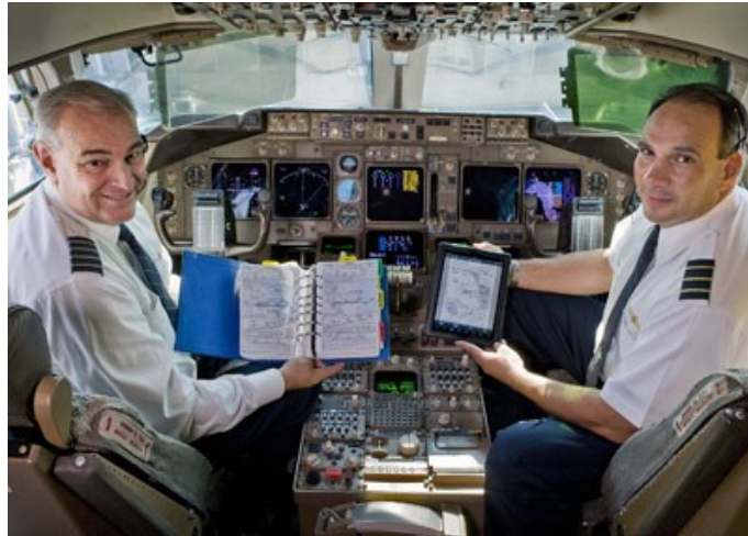
Figure 8.3.: Figure 8.3 shows United Airlines pilots using a light weight tablet device in order to replace 38 pounds of operating manuals, navigation charts, reference handbooks, flight checklists, logbooks and weather information found in pilot bag. Source: 88.
