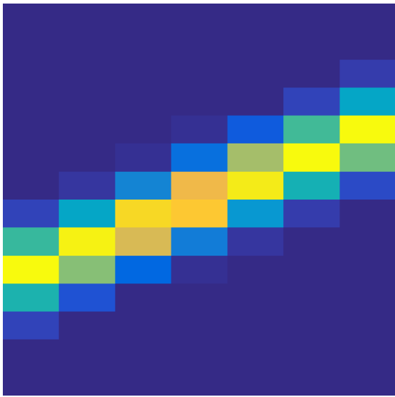
(c) Response map generated with the STFT with a relatively large window.
