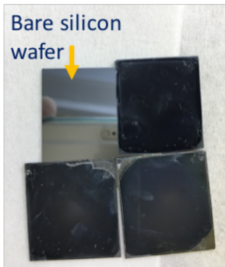
Figure 6.9. Comparison of silicon wafer before and after processing with metal salt : polymer composite film and DRIE. It can be seen by eye how they show less reflectivity with respect to bare silicon wafer.
