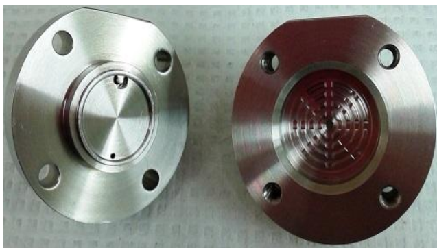
Figure 15: Internal structure of the membrane holder used for the experiments
