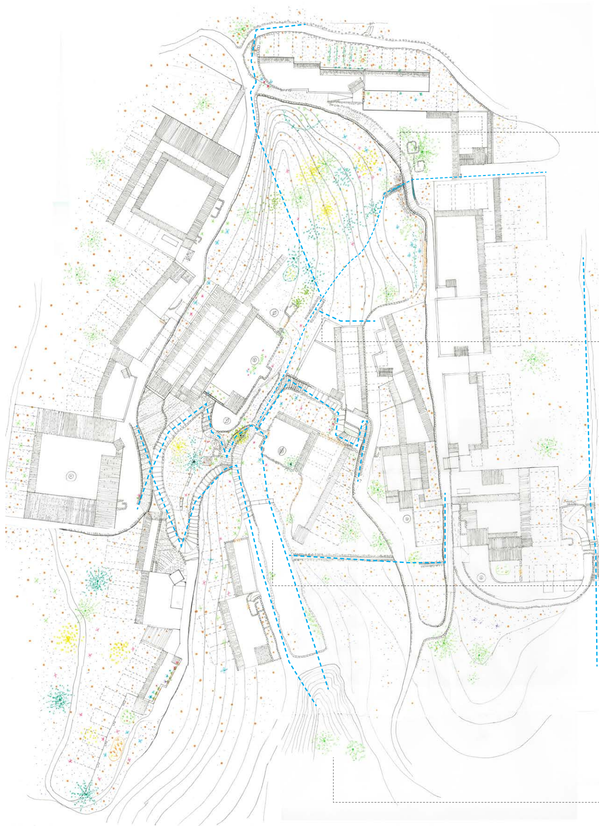
FIG 6.12 Li-family-mountain Village drainage plan
