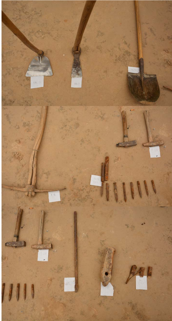
FIG 3.5 Yao-dong construction tools in Mizhi
