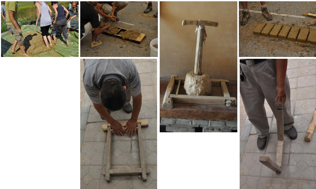
FIG 3.63 Wood module used to make adobe (Ren-ma-zai village, and Bei-ying Folk Museum, Henan)
