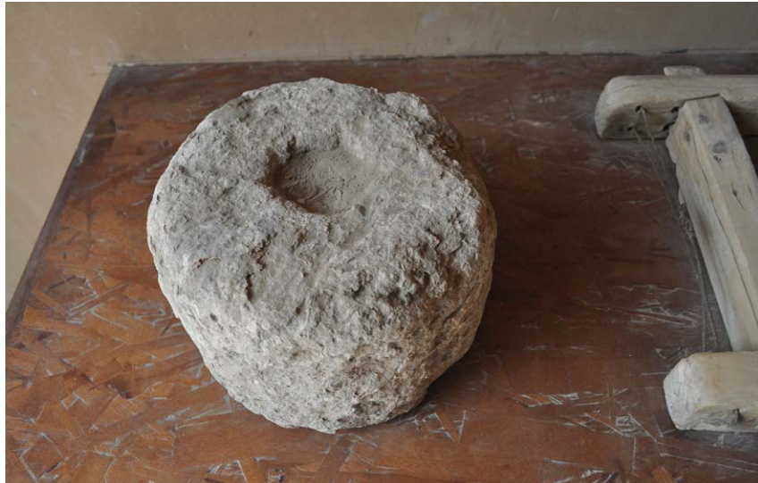
FIG 3.62 A stone attached to a handle, used to compress the soil into an adobe brick. (Bei-ying Folk Museum, Henan)
