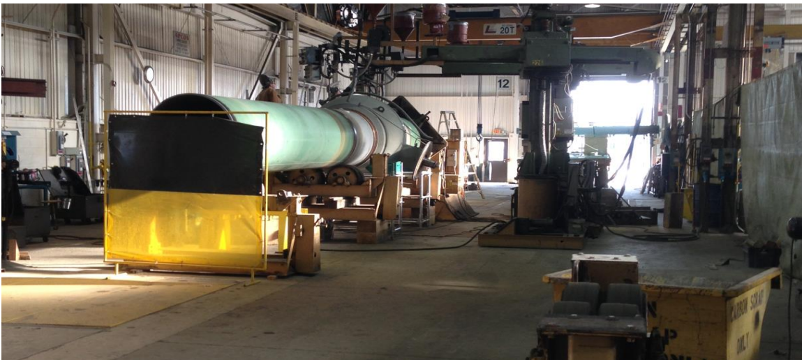
Figure 2-2: Large diameter pipe spool fabrication in piping fabrication facility, Cambridge, Ontario
