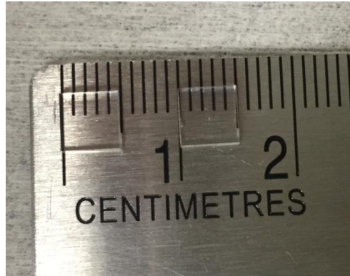
Figure 3.2 Quartz dummy chips used in electrical property measurements of sintered silver.
