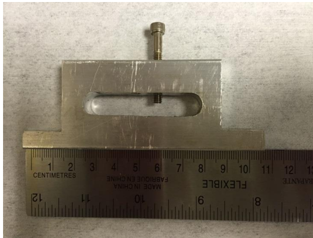
Figure 3.9 Fixture used to apply pressure via screw during production of Group C and D samples.
