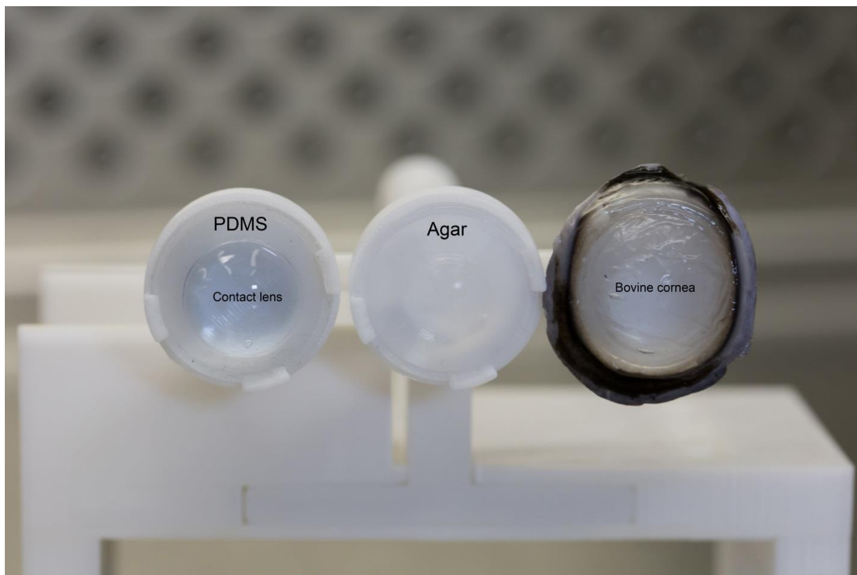
Figure 6-4 Sample eyepieces: Sample of PDMS eye piece with a contact lens, an agar eye piece, and ex-vivo bovine cornea mounted eye piece
