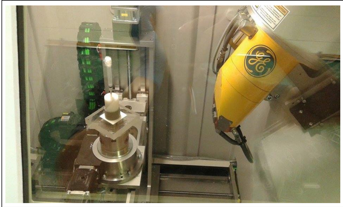
Fig (4.11) Hydrogel sample injected with water and subjected to beams of X-ray to create 3-D images of the cavity expansion.
