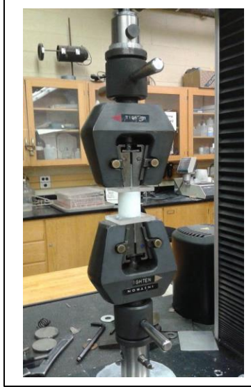
Fig (4.3) PVA hydrogel sample mounted between two flat plates during unconfined compression test.
