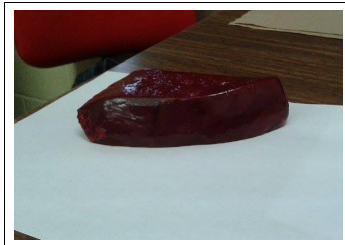
Fig (6.3) Sample of spherical expansion test.
