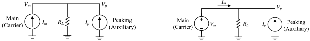
(a) Initial realization of load modulation with two VCCSs. (b) modified circuit with the main VCCS replaced by a VCVS.
