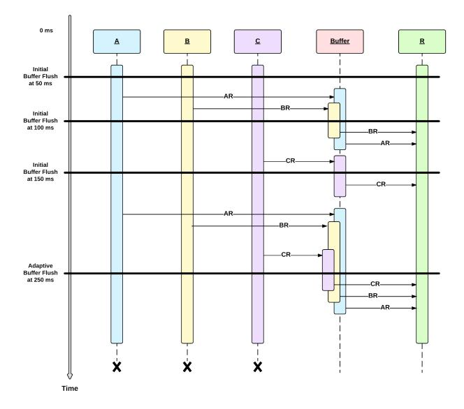
Figure 3.8: An example of adaptive buffering method for reordering messages.
