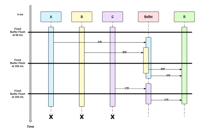
Figure 3.6: An example of buffering method which does partial reordering.
