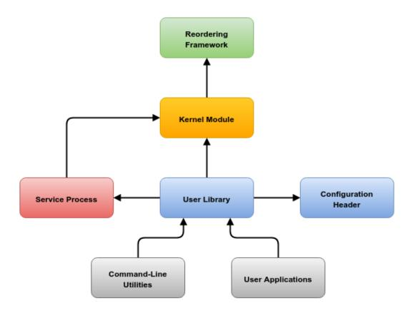
Figure 5.1: The reordering framework architecture.
