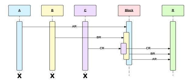
Figure 3.4: An example of blocking method for reordering messages.
