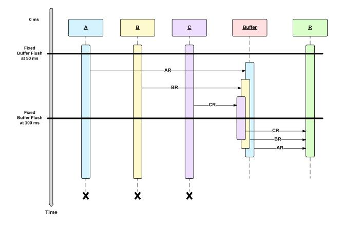
Figure 3.5: An example of buffering method for reordering messages.
