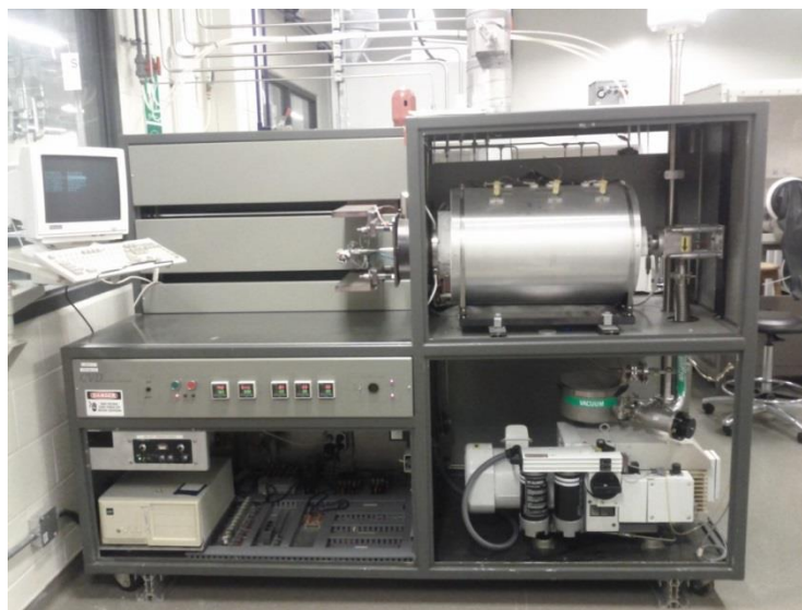
Figure 3-1 Image of the LPCVD system used for growth of ZnO NWs
