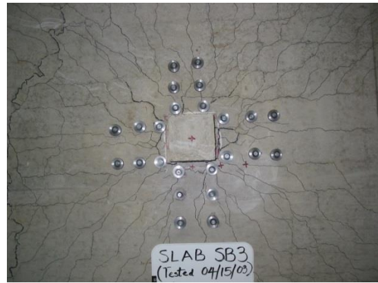
b) SB3 slab (Cracking from FEA and test)
