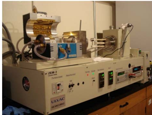
Figure 3.15 ZEM-3 Model M8 measuring from room temperature up to 800°C, using thermocouple probe type R and electrode type Ni.
