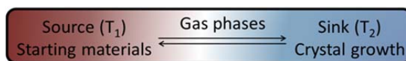
Figure 3.4 (a) Schematic illustration of chemical vapor transport; (b) Reaction tube inside a two zone furnace for chemical vapor transport.
