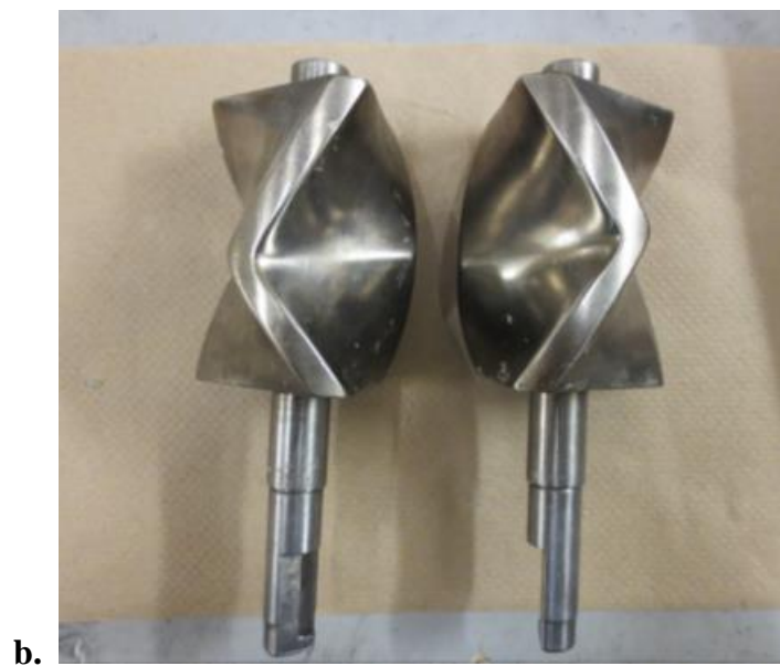
Fig.3.2 The HAAKE batch mixer system: (a.) Rheocord 90 equipped with RHEOMIX 3000, (b.) roller-blade rotors employed for mixing.
