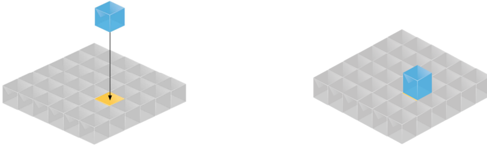
Figure 3-4. Execution of an adsorption event on the lattice by picking a site and adding an atom on top of that lattice site.
