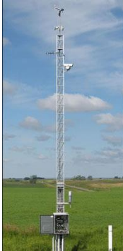
Figure 2.1 - Typical RWIS Station with Environmental Sensors (North Dakota Department of Transportation, n.d.)
