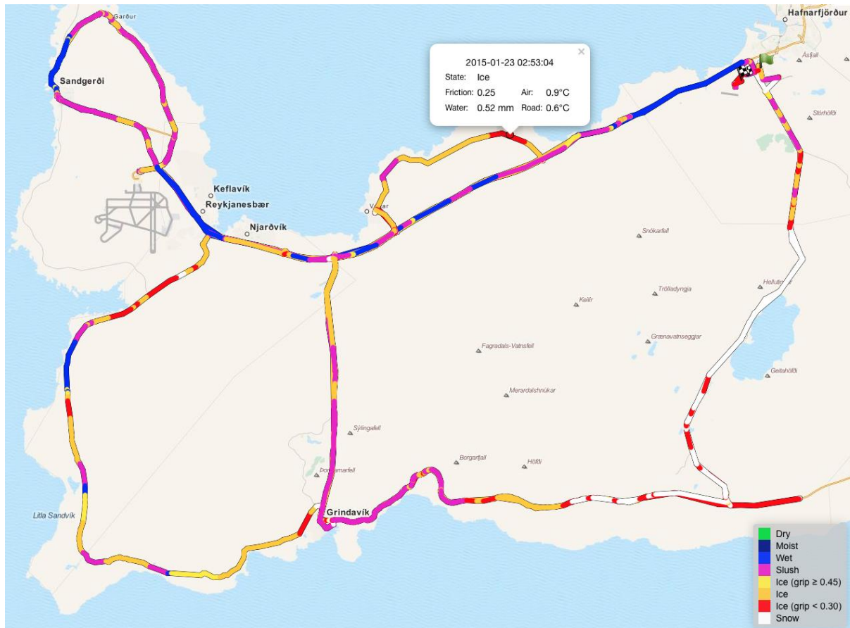
Figure 2.5 – RCM411 Spectroscopic Data on Map (Teconer, n.d.)
