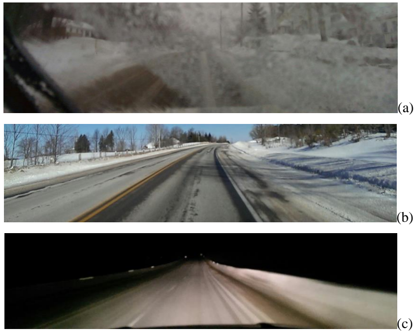
Figure 3.5 - Sample Images of Key Performance Factors: (a) Image with poor visibility (b) Dried residual salt on road surface (c) Image captured in night-time
