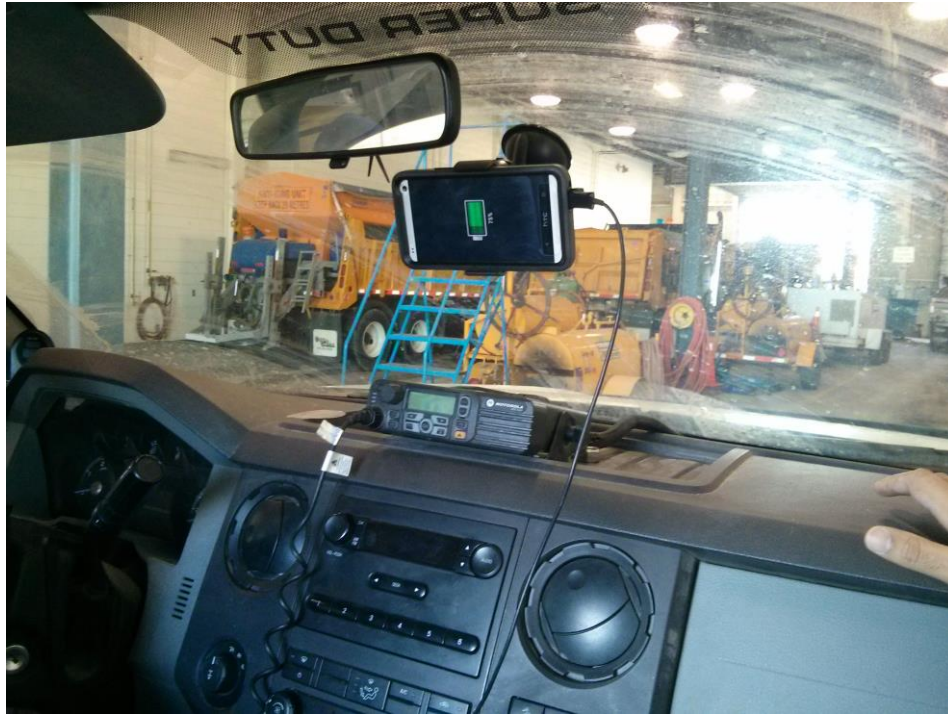
Figure 2.11 - AVL-Genius Device - Smartphone and Control Box
