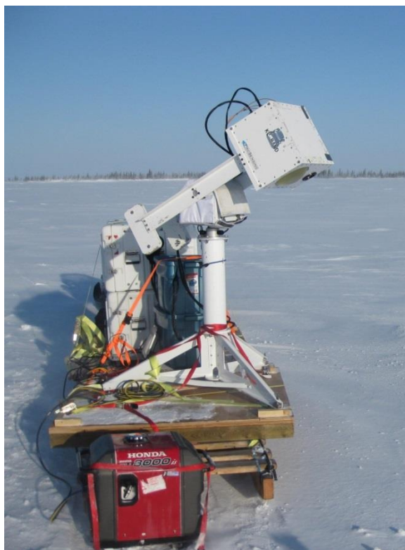
Figure 3-12: Sled-borne UW-Scat field set up during Ku-band scan of undisturbed static site on Malcolm Ramsay Lake near Churchill, Manitoba.
