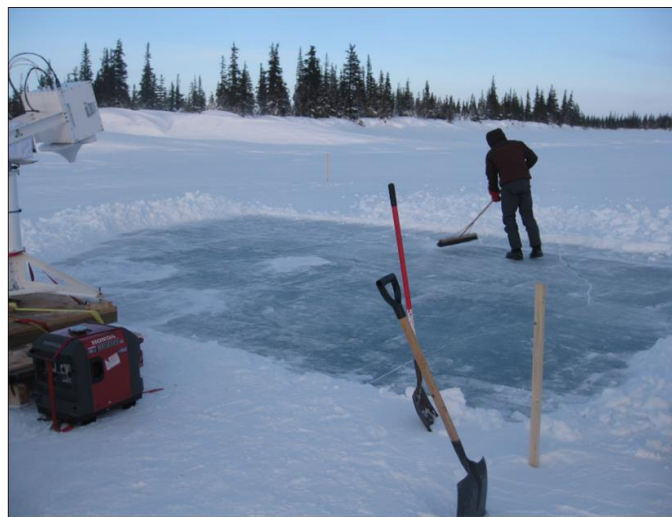
Figure 4-7: Procedure of snow removal from the scatterometer field of view at completion of the observation period at Site 1 (March 5, 2011).
