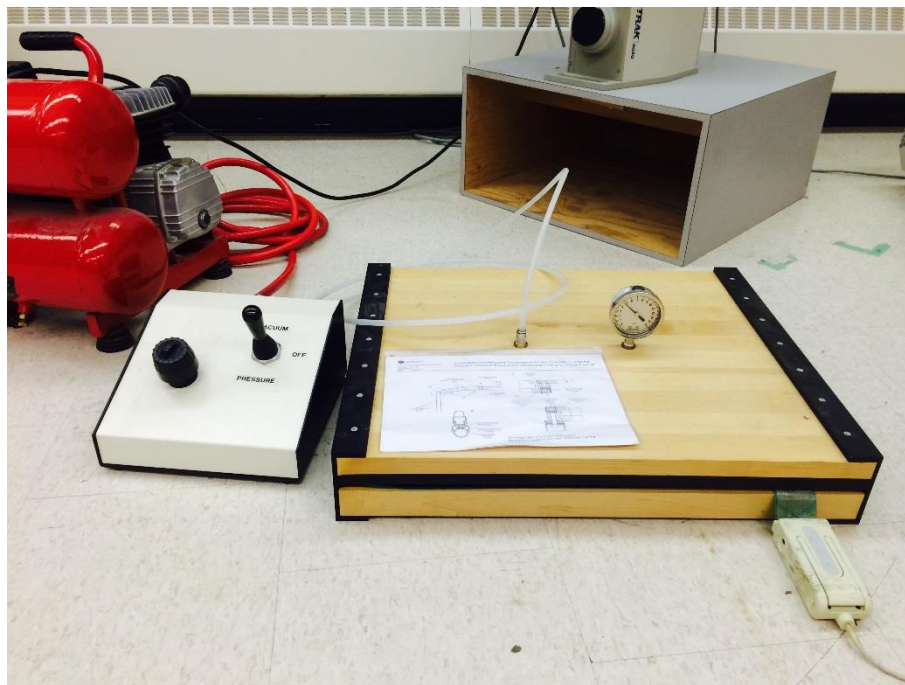
Figure A-1: Calibration and equilibration equipment showing the air compressor, control panel and pressure mat in the wooden scaffold.
