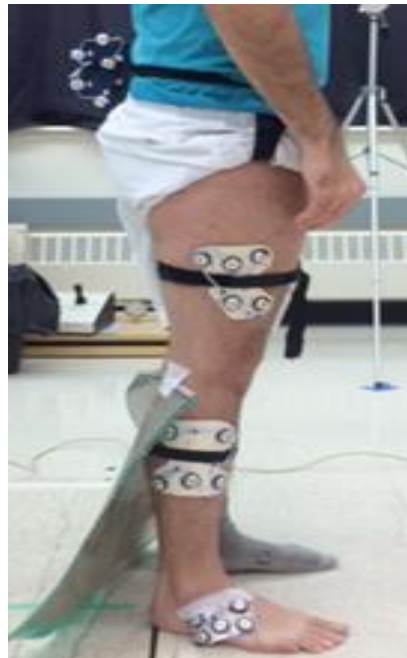
Figure 3-1: Experimental set-up used in this investigation. The pelvis, thigh, shank and foot marker clusters are visible as well as the pressure mat attached just below the popliteal crease on the participant's calf.
